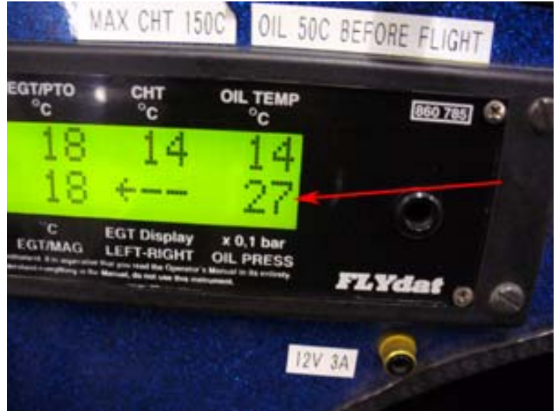
Figure 21: Flydat showing 2.7 bar oil pressure
