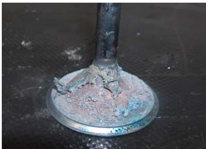
Figure 8: Valve after 1000 hours Avgas use
