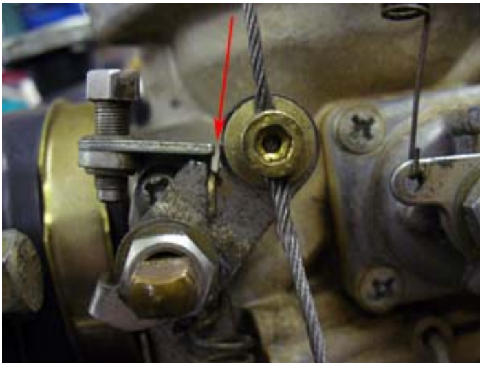
Figure 40: Throttle lever with clearance at full throttle
