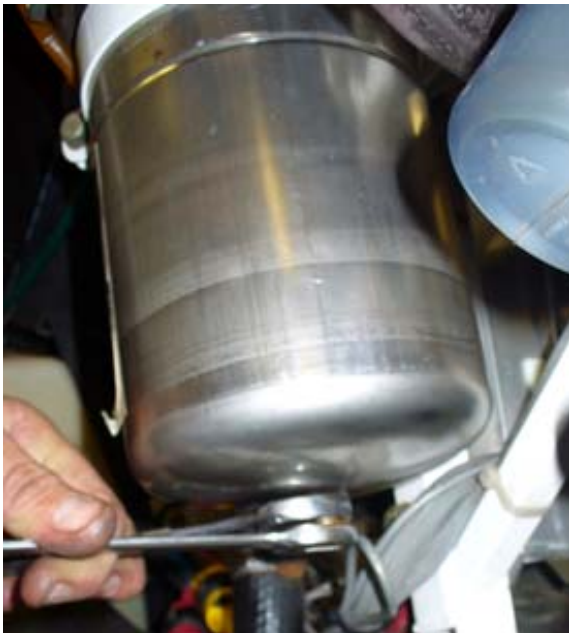
Figure 18: Undoing oil tank drain bung
