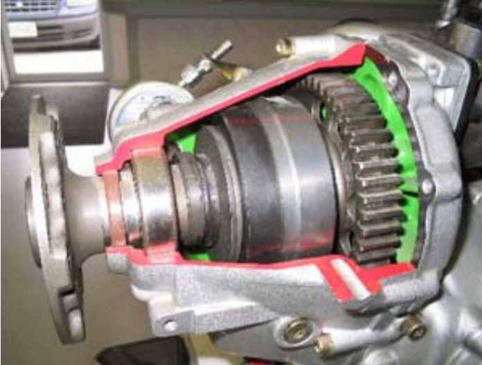
Figure 44: Gearbox with slipper clutch
