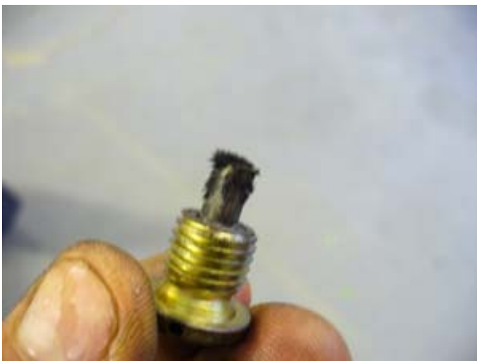
Figure 31: Plug after cleaning in carb cleaner
