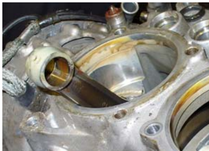
Figure 9: White lead deposits from Avgas on top of conrod
