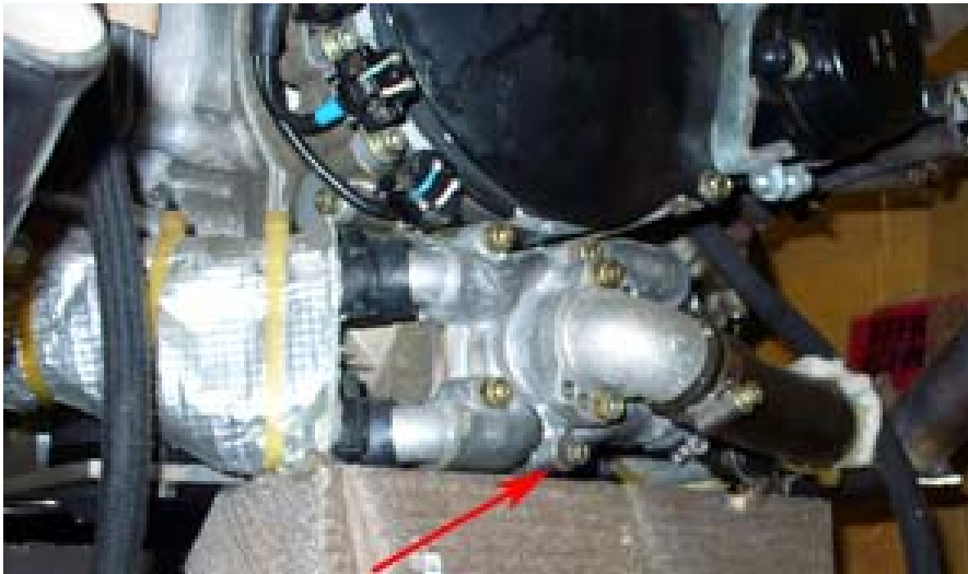
Figure 52: Water drain screw on water pump
