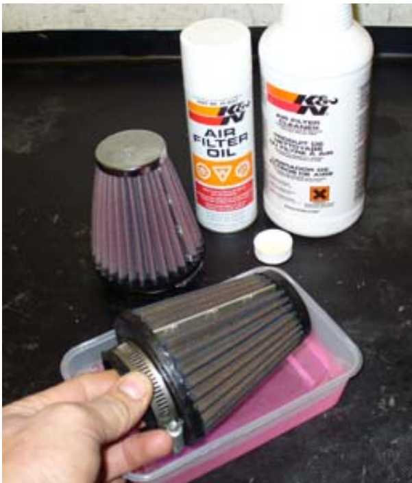
Figure 43: Clean air filter shown with dirty filter about to be cleaned
