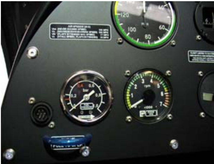
Figure 11: Fuel pressure gauge fitted
