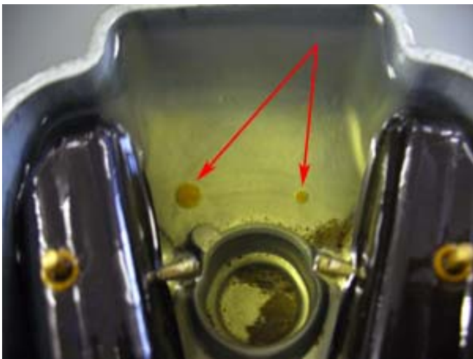
Figure 36: Water in the float bowl
