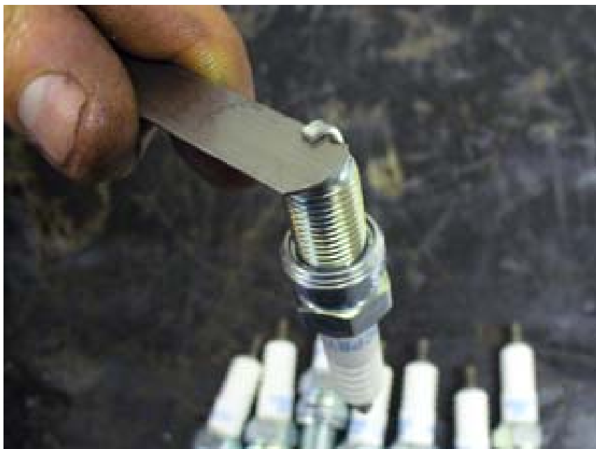
Figure 33: Checking plug gaps before installation
