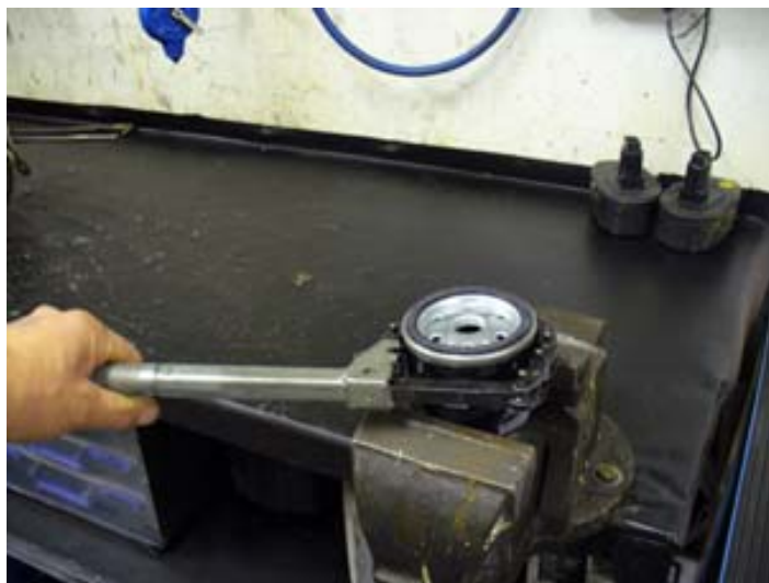
Figure 23: Cutting open the filter
