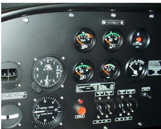
Figure 3: Instrument marking kit fitted to a Eurostar
