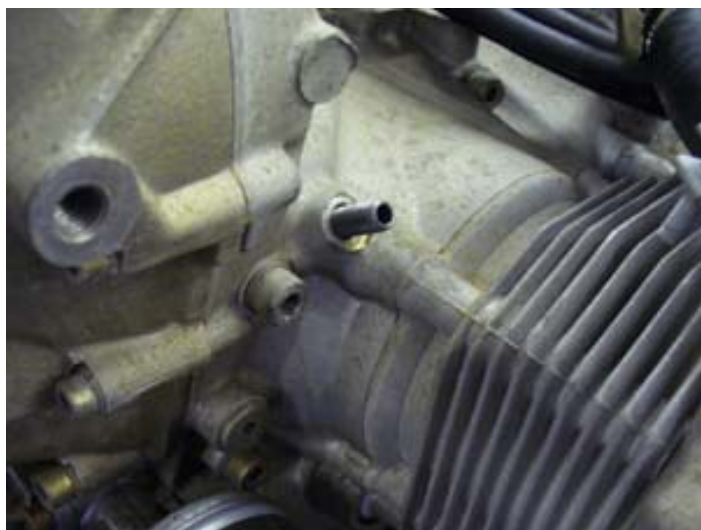
Figure 48: Crankshaft locking pin location
