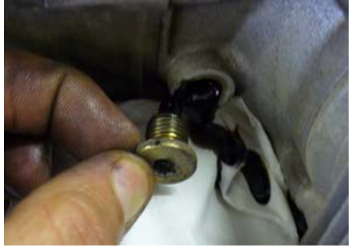
Figure 28: Oil behind magnetic plug
