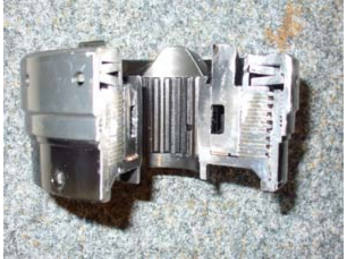
Figure 45: Cut away of slipper clutch
