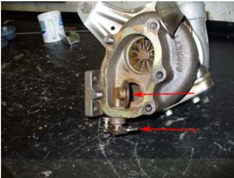
Figure 17: Inside of turbo showing waste gate and control lever
