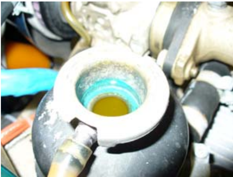
Figure 16: Corroded expansion tank
