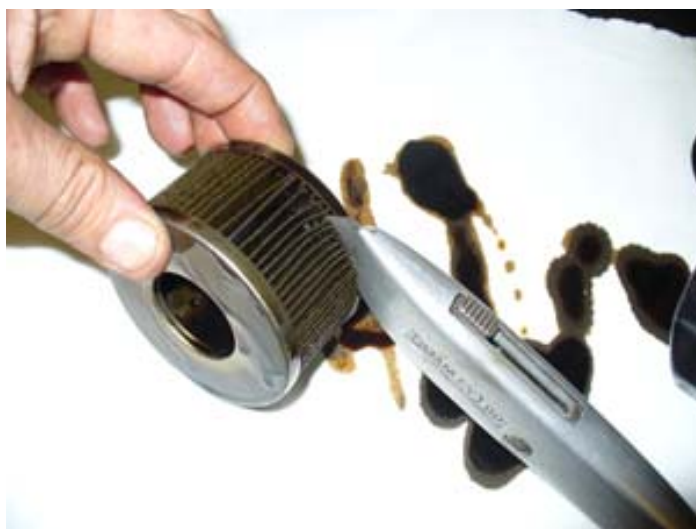
Figure 24: Removing the filter paper.
