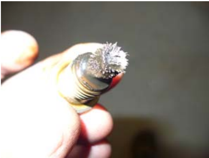
Figure 29: furred magnetic plug before cleaning
