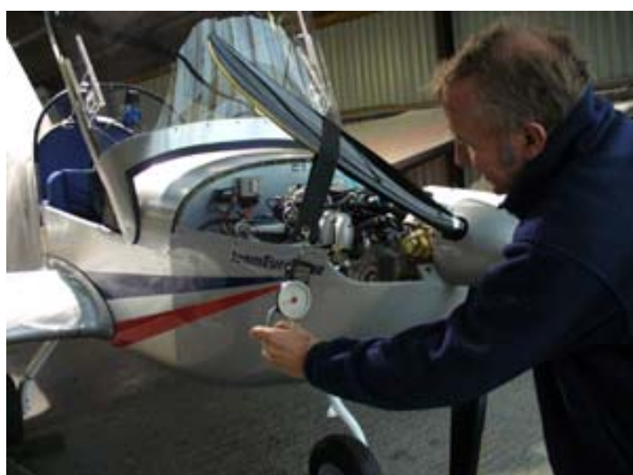
Figure 49: measuring friction torque at 1/2 m on the prop
