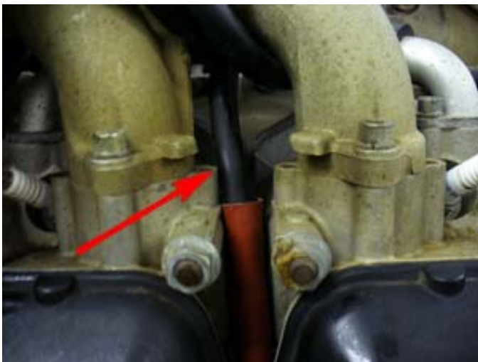
Figure 12: HT leads fretting on head due to poorly positioned sleeve
