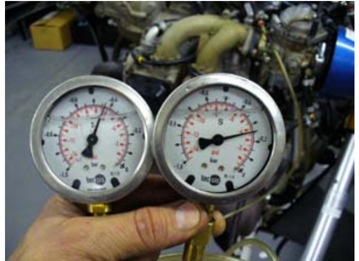
Figure 42: Pneumatic carb balancers
