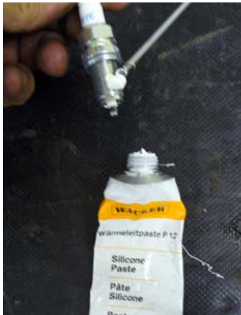
Figure 32: Applying heat sink paste
