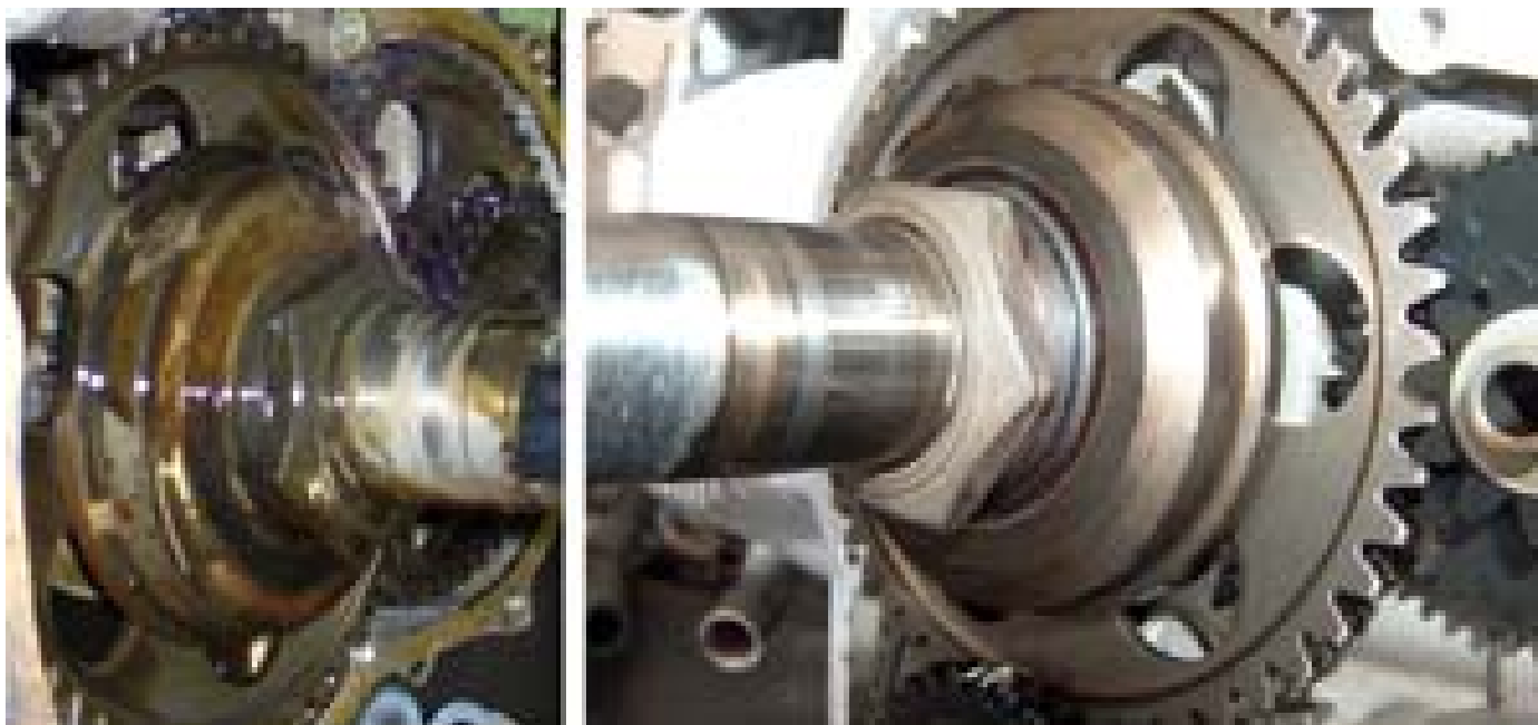
Figure 7: Sprag clutch in an engine run on Avgas (left) and the same component in an engine run on Unleaded Mogas
