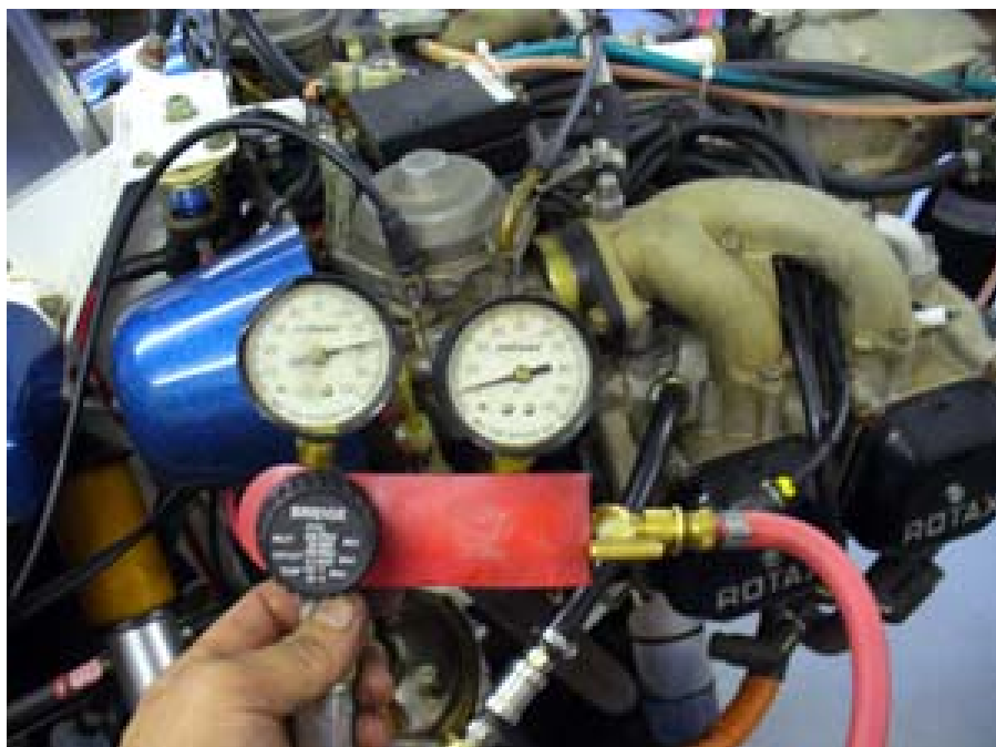
Figure 51: Leak down (differential) compression tester
