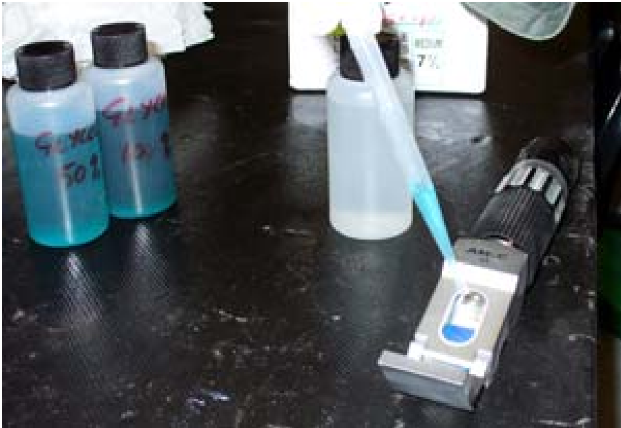
Figure 14: Using refractometer to check glycol ratio
