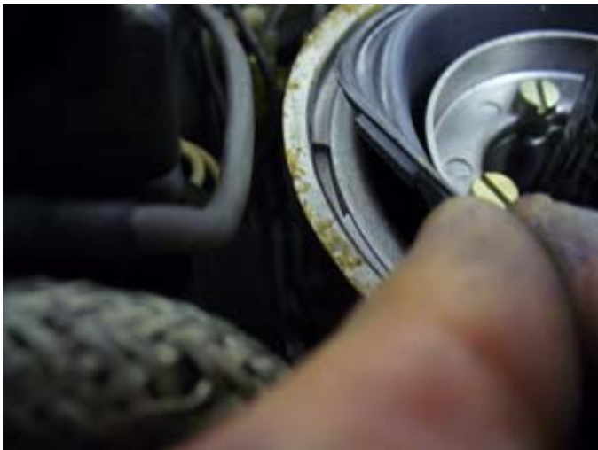
Figure 38: Diaphragm location lug and recess.
