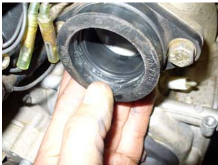
Figure 39: Checking carb rubber flange for cracks
