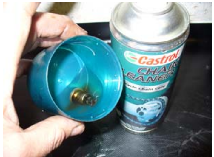
Figure 30: Cleaning magnetic plug
