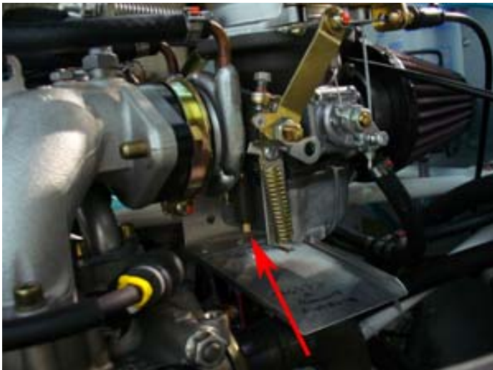
Figure 41: Photo 37 of idle mixture screw (hex).
