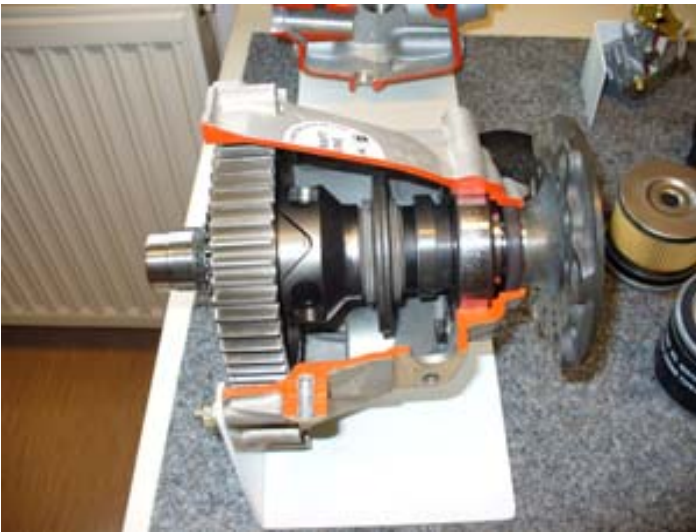
Figure 47: Gearbox without slipper clutch
