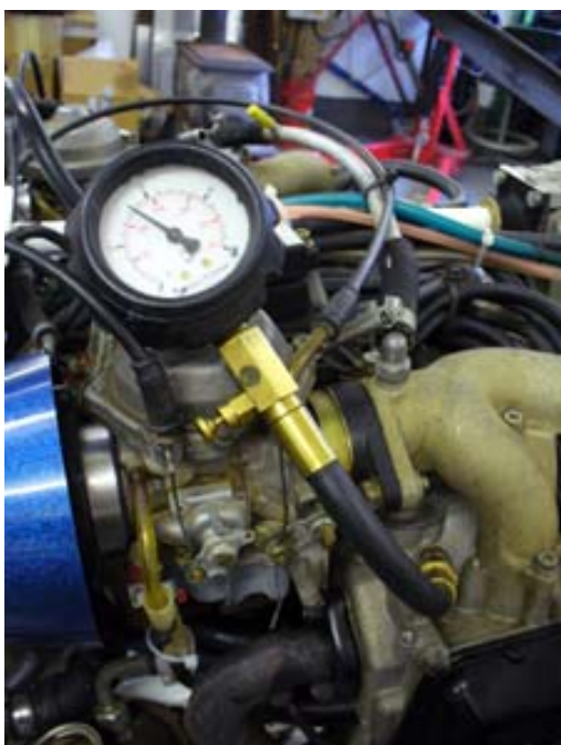
Figure 50: Conventional automotive style compression tester
